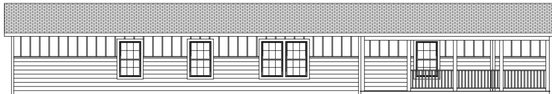
OPT. LAP & VERTICAL BOARD & BATT EXTERIOR
